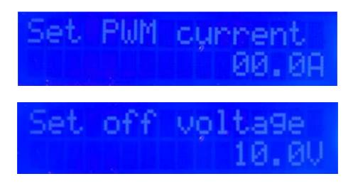
Using the **Right side** parameters you can set Current and Voltage levels how much current do you want in your HHO cell and where do you want the controller to switch the relay driver output ON/OFF.
